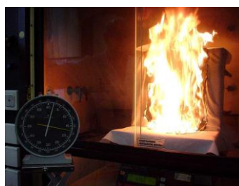
(b) BS5852, Crib 5. Fire in case of a failed test
