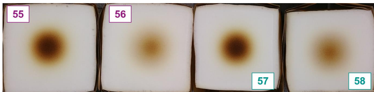
Figure 10. Scorching test of two pairs of foams made according to formulation 3. Reduction of the index and an addition of ORTEGOL® HA1 to maintain hardness led to a significant reduction of scorch (microwave irradiation: 80 s, 1000 W).
